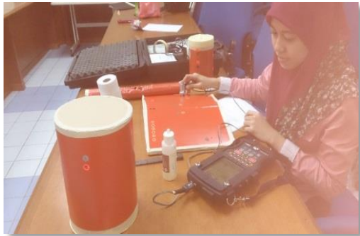
Ultrasonic tester from Nuclear Malaysia performing ultrasonic testing during PTP
